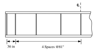
Figure 3.14 : Spacing of Intermediate stiffeners
