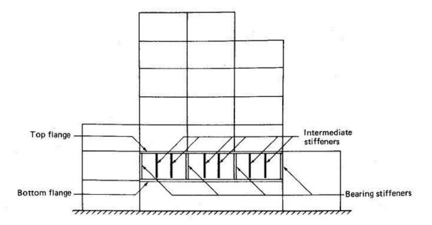
Figure 3.1: Plate girder in a multistory building
