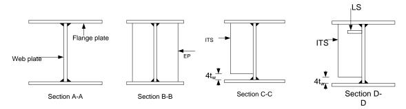
Figure 3.4(d): Forms of plate girder
