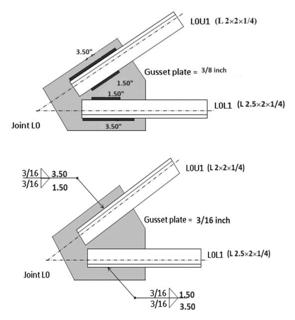
Figure 2.22: Weld design of joint L<sub>0</sub>
