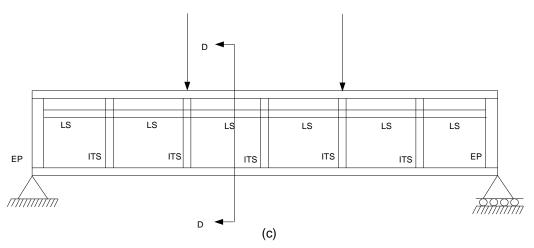
Figure 3.4(c): Plate girder with intermediate, bearing and lateral stiffeners
