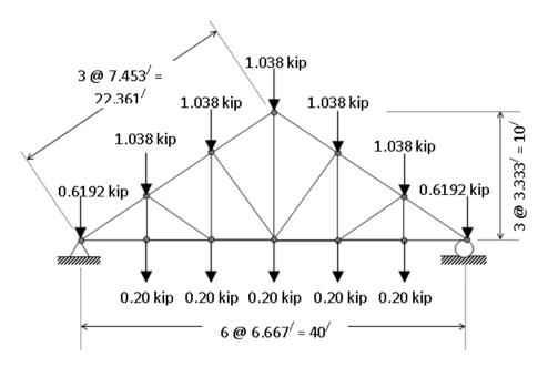
Figure 2.13: Dead loads on the truss
