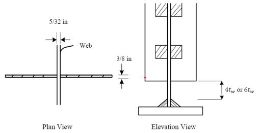
Figure 3.15: Plan and Elevation View of Intermediate Stiffeners
