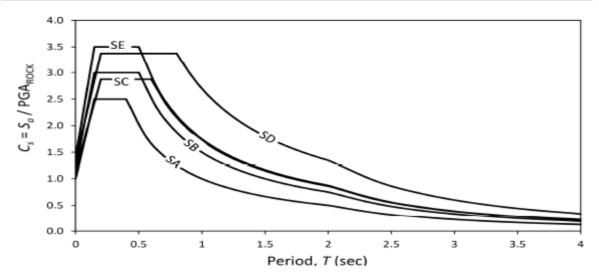
Figure 6.2.26 Normalized design acceleration response spectrum for different site classes.
