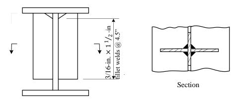
Figure 3.19: Weld between web and intermediate stiffener
