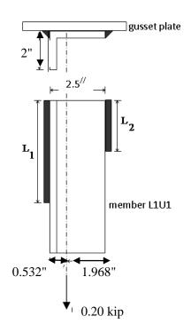
Figure 2.25: Weld design of member L<sub>1</sub>U<sub>1</sub>
