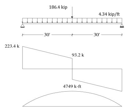
Figure 3.12: SFD and BMD for the recomputed factored loads
