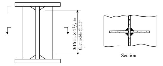
Figure 3.20: Weld between web and bearing stiffener
