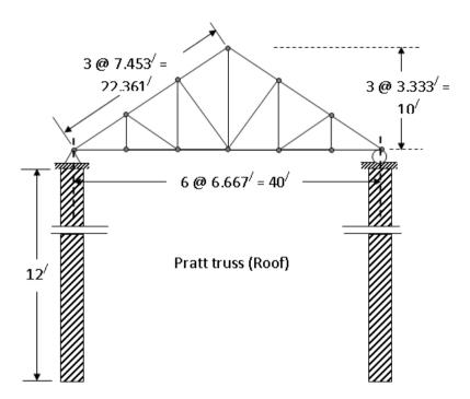
**Figure 2.5: Pratt type Roof Truss**
