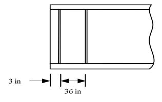
Figure 3.17: Side view of the plate girder
