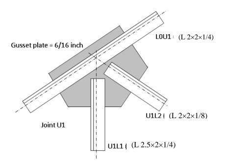
Figure 2.23: Weld design of joint U1
