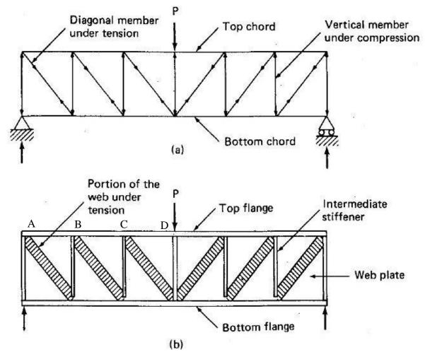
Figure 3.5: Analogy between a truss and a stiffened plate girder
