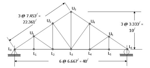
Figure 2.11: Truss notations (member numbering): Pratt truss (Roof)
