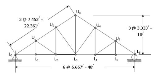
Figure 2.6: Truss notations (member numbering): Pratt truss (Roof)
