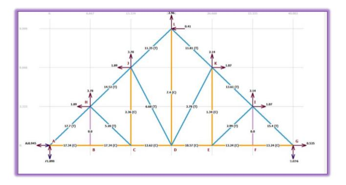
Figure 2.16: Wind loads on the truss for wind blowing from left to right
