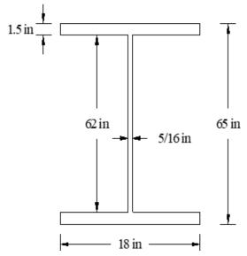
Figure 3.11: Cross-section of the plate
