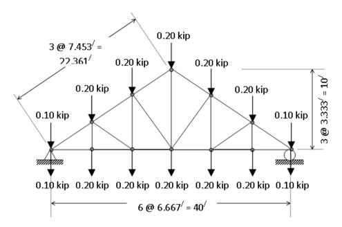
Figure 2.12(a): Dead loads on the truss (self-weight distribution)
