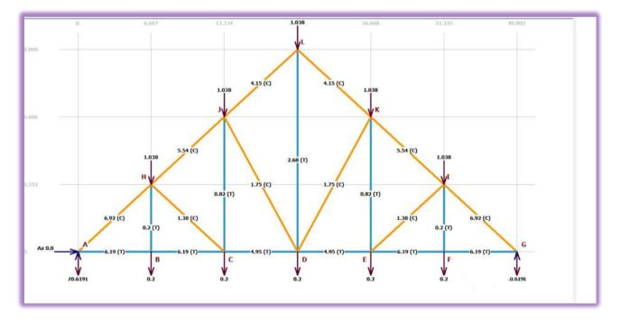
Figure 2.18: Dead loads on the truss
