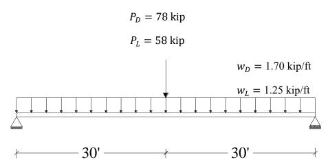
Figure 3.8: Plate girder to be designed under service loads
