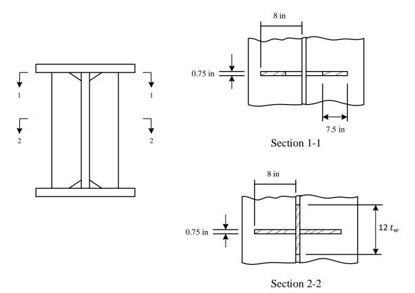
Figure 3.16: Bearing Stiffener at the Support
