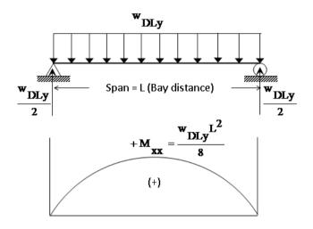
Figure 2.8: Bending moment diagram for loading in Y direction (loading perpendicular to the roof surface, bending parallel to the roof)
