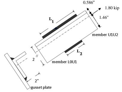
Figure 2.24: Weld design of member L<sub>0</sub>U<sub>1</sub> and U<sub>1</sub>U<sub>2</sub>
