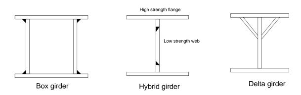
Figure 3.3: Types of plate girder
