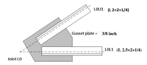
Figure 2.19: Joint Lo of roof truss
