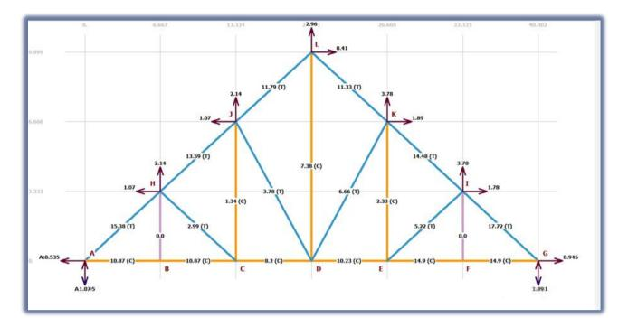
Figure 2.17: Wind loads on the truss for wind blowing from right to left
