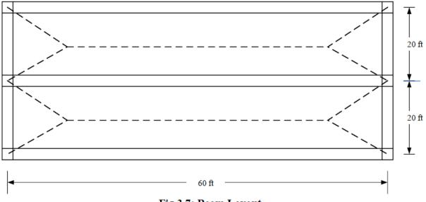
Fig 3.7: Beam Layout
