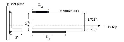
Figure 2.20: Weld design for L<sub>0</sub>L<sub>1</sub>
