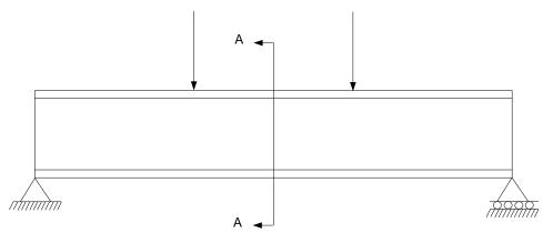
(a) Figure 3.4(a): Plate girder without stiffeners
