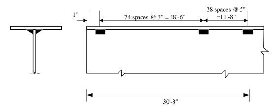
Figure 3.18: Weld between Flange and web
