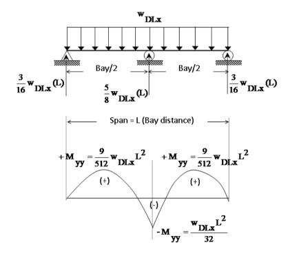
Figure 2.9: Bending moment diagram for loading in X direction (loading parallel to the roof surface, bending perpendicular to the roof)
